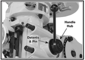
Figure 38. Coarse downfeed handle hub, detents, and pin.
